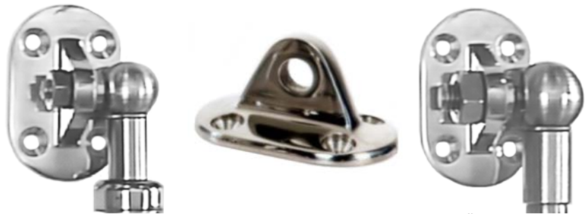
#64.088 Hatch mounting bracket: 1 1/2" x 2 3/8" footprint 3/4" stand off Showing M8 ball joint #62.830 to be ordered separately #64.098 for M10
